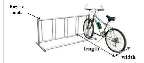
The rectangular floor area that are required for the parking of the bicycles is determined by considering the following:
