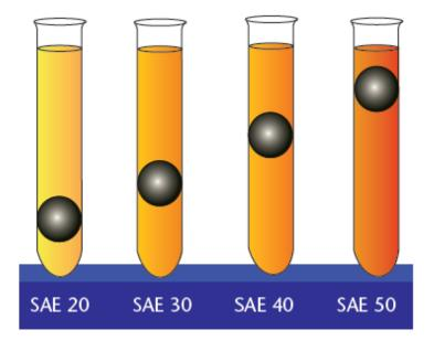
Which SAE represents an engine oil with a higher viscosity?
