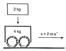
4.1.1 Calculate the velocity of the trolley and brick after the brick has fallen on the trolley.
