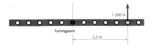
5.3 Use the sketch hereby to determine the magnitude of the unknown force at A which balances a weightless beam.
